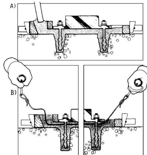
Diagram A illustrates the use of grout surcharge to ensure complete filling under a base.
